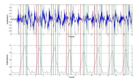
FIGURE 2. Knee sound signals segmented "up" and "down" during 25° to 75° of flexion.
