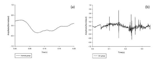
FIGURE 3. (a) VAG signals from one normal knee and (b) sound signals from abnormal knee. The recording system used was set in the same condition for recording these two signals. Abbreviation: VAG: vibroarthrographic;
