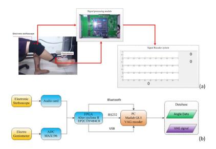
FIGURE 1. (a) Knee flexed  $(90^{\circ})$  and fully extended  $(0^{\circ})$  in a sitting position as measured with a goniometer. (b) An overview of the VAG signals recording system flowchart.
