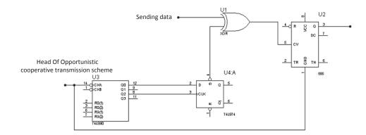
FIGURE 12. Implementation of circuit signal modulation
