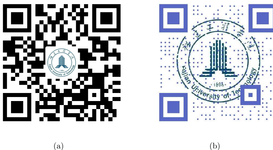
FIGURE 3. QR code visual improvement method. (a) The logo embedded method which covers a small logo in the center of QR code; (b) A picture is added to the entire QR code region as a background.
