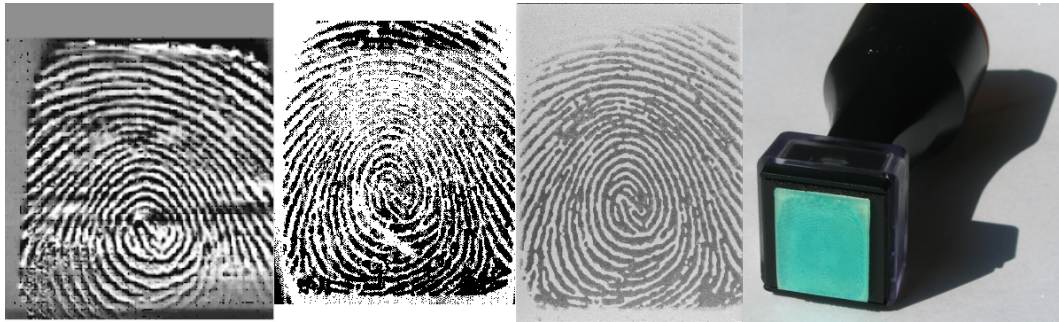
FIGURE 1. The stamp captured by thermal fingerprint sensor Bergdata FCAT 100 (left fingerprint), by optical fingerprint sensor Suprema SFM3020-OP (middle fingerprint) and by capacitive fingerprint sensor Suprema SFM3050-TC1 (right fingerprint). Picture of the stamp (right picture). [5].
