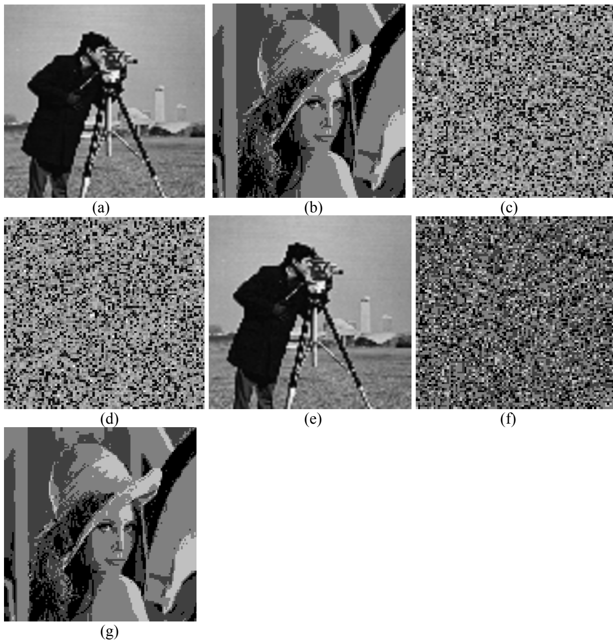
FIGURE 2. (a) The original Cameraman image, (b) the two most significant bits of Lena as the watermark, (c) the rearranged image of Cameraman using Algorithm 3.1, (d) the watermarked image of the rearranged image using LSB substitution, (e) the rearranged back of the preceding watermarked image using Algorithm 3.2, (f) the extracted 2 bits of LSB (g) the rearranged back of the preceding extracted image using Algorithm 3.2.
