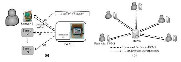
FIGURE 2. (a) Polling commands between a transmission unit and sensors; (b) A service scenario of HCMS.
