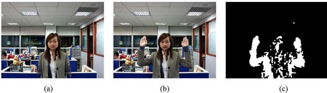
FIGURE 4. Illustration of foreground segmentation: (a) background model before hands up, (b) current frame while hands up, (c) foreground of current frame
