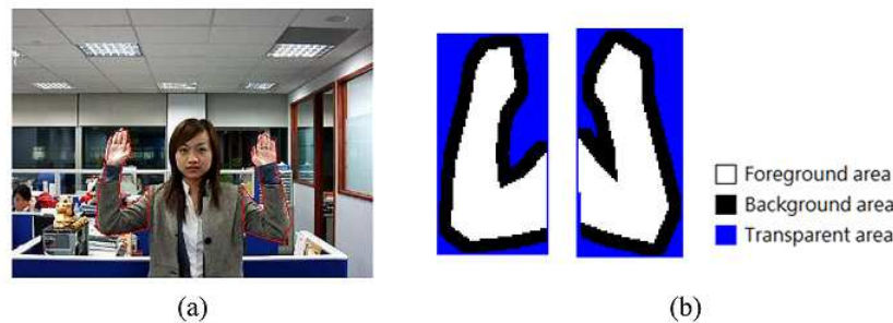
FIGURE 7. Template building: (a) manual segmentation of two arms when hands up, (b) left- and right-arm templates from the segmentation
