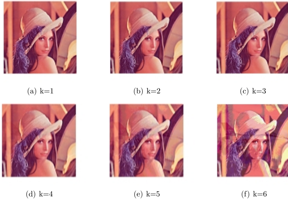
FIGURE 1. Stego image of hiding Airplane image in lena cover image with k LSBs from 1 to 6
