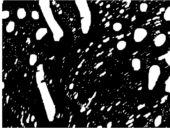
FIGURE 6. The re-shaping and merging of catchment basin markers
