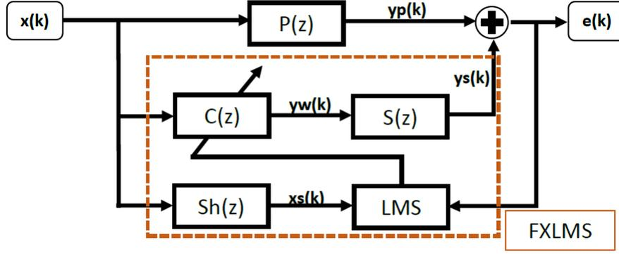
FIGURE 1. Block diagram of FxLMS algorithm.
