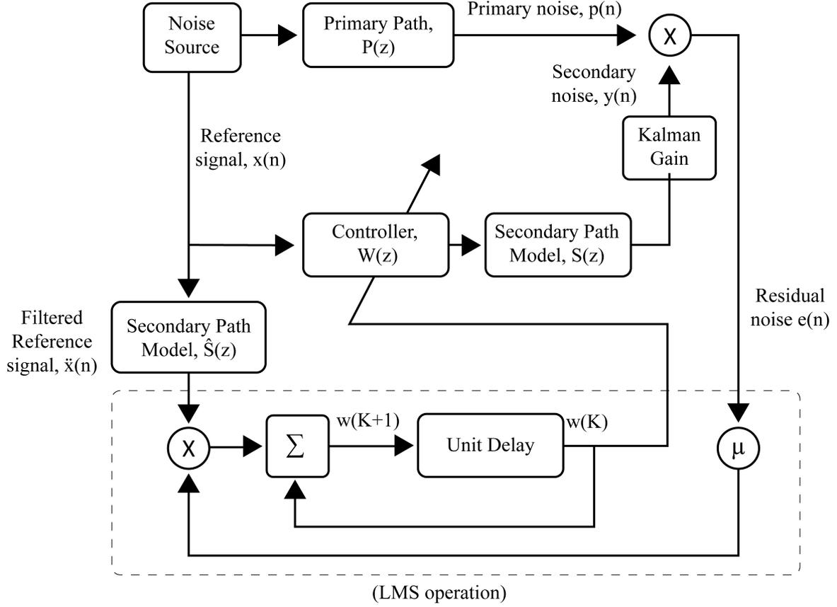
FIGURE 3. Modified FxLMS algorithm.
