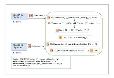
FIGURE 2. The Communication Process within the CCM Scheme
